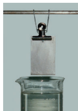
DAIPALITE-Ei A / Ei Almost no corrosion
