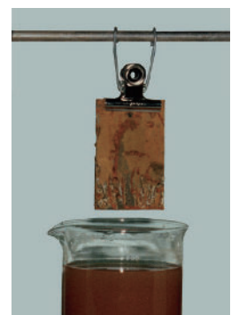
Rock wool Many Corrosion of about 600µm depth can be seen.
